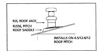
FIG. J - 90-RJS56 ROOF SADDLE, HI PITCH ROOF
